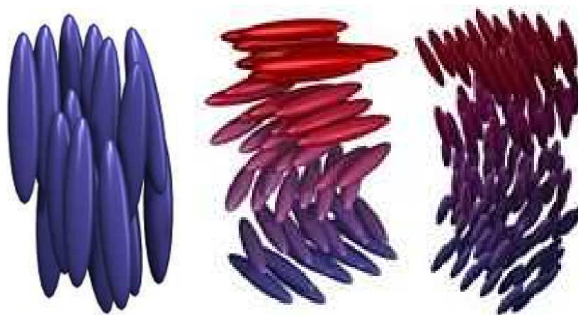
Figure 6.3: Nematic (left) and cholesteric phases (middle and right) for a calamitic liquid crystal [44]. The phase shown on the right is called smectic C*, where the molecules are arranged in layers, and the tilt angle varies from layer to layer.
