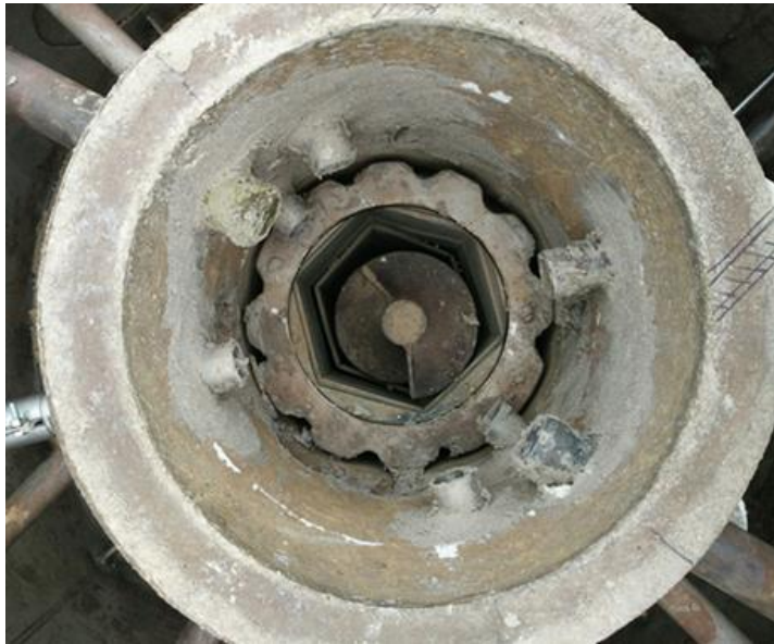
Fig. 4 Lining of the reactor with a movable grate
