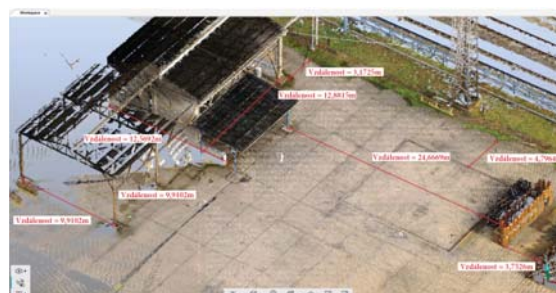
Fig. 2 3D view of the entire project with a demonstration of dimensional measurement (Nejtková and Marek, 2017)
