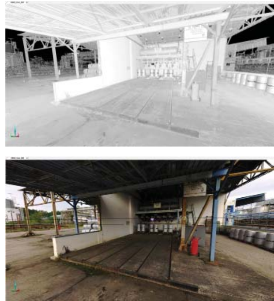
Fig. 1 Detail of an infrared and colour scan of a loading station with marked scanning positions (Nejtkova and Marek, 2016)
