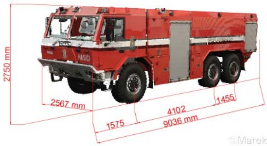
Fig. 9 Acquired true and accurate special coloured model of the fire engine with simple dimension capability example
