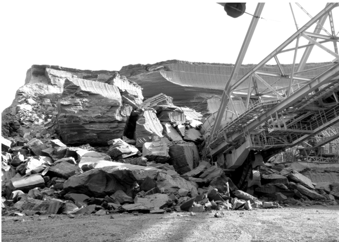
Fig. 6 Sudden landslide or rockslide could damage the excavator (Most Basin, Bilina Quarry on 11 May 2009).
