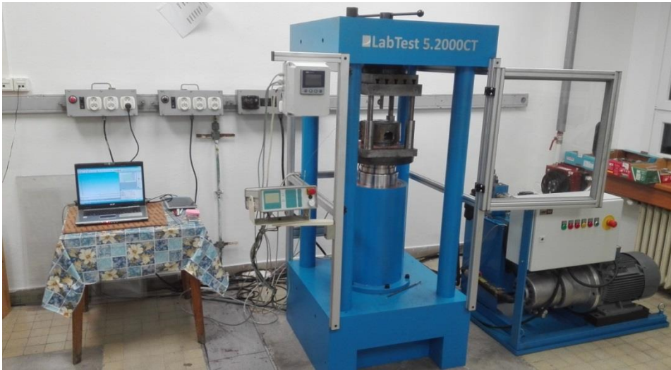
Fig. 3 Workplace of VŠB-TUO for materials forming by ECAP method
