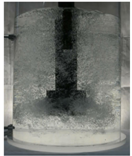
c) Variant C: 350 rpm and 15.0 \text{Nl}\cdot\text{min}^{-1}
