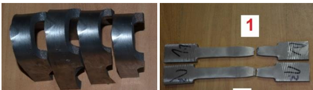
Fig. 4. Test rods for weld bending test (left) and transverse tensile test (right)
