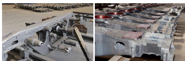
Fig. 1. Parts of wagon chassis made of cast steel [11]
