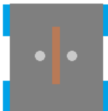
Fig. 4.2: Robot with two phototransistors (light grey) divided by barrier (brown).
