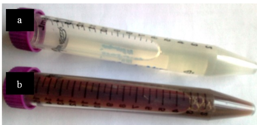
Figure 10: An illustration photo (a) leachate of Tilia sp. and (b) colloid of Ag NPs 24 hours after mixing the plant leachate with aqueous solution of AgNO 3 .
