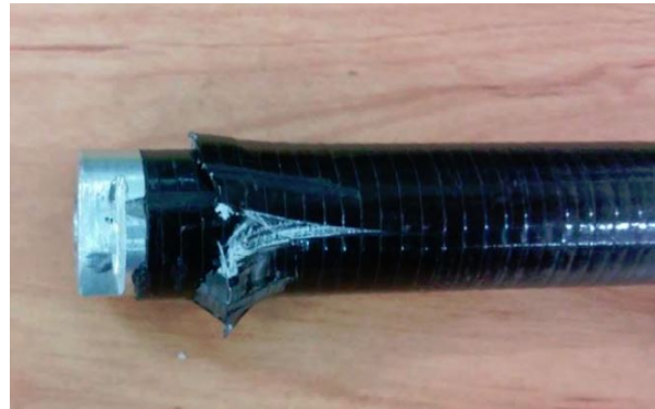
(b) Closer look to the specimen's broken area
