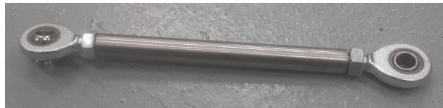
Figure 4.5: Rod replacing dampers
