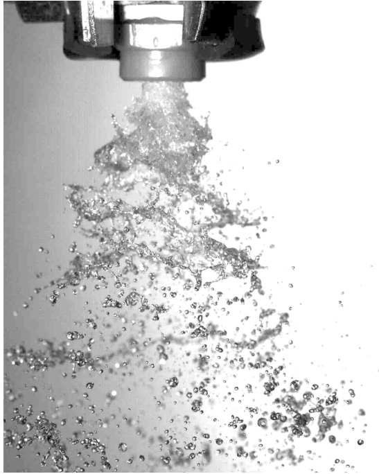
Figure 8.3: High-speed camera image of water nozzle (type 90B2FP6.5).
