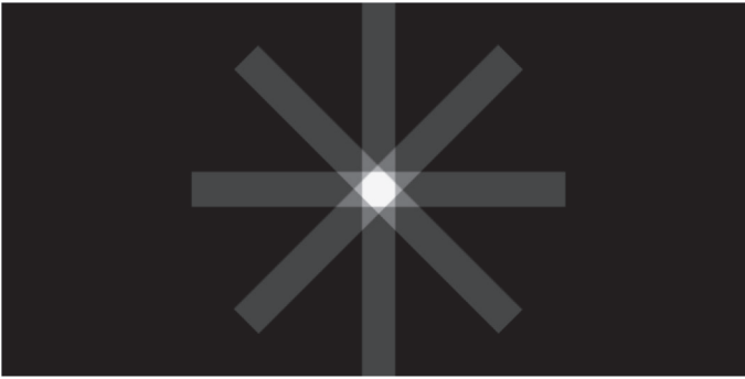
Fig. 3 Reconstructed object with the star artefact.
