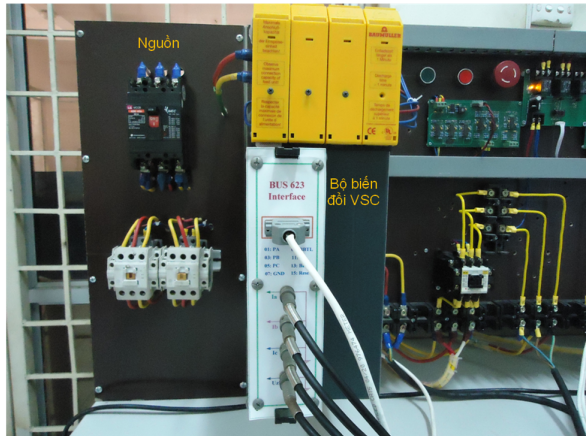
Fig. 17: The VSC converter using Baumuller Servo-Power-Unit BUS 621, 622, 623, 624; nominal voltage 600V, nominal current 20 A.
