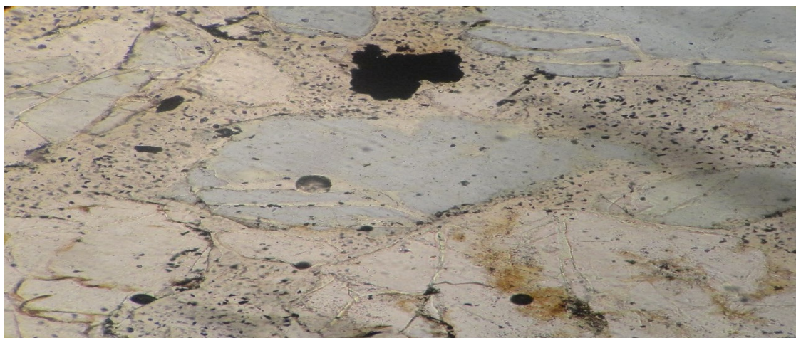
Plate 2: Photomicrograph of a coarse grained sandstone in plane polarised light.
