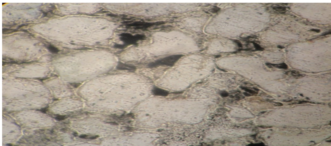
Plate 1: Photomicrograph of a medium grained sandstone in plane polarised light.
