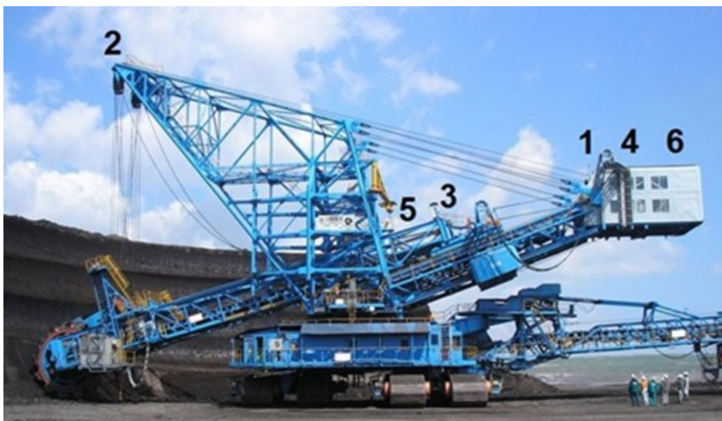
Fig. 2 Excavator K800 (legend: GNSS receivers (GPS1, GPS2), 3 IRC, 4, 5 inclinometers, 6 evaluation unit, K wheel axis centre)
