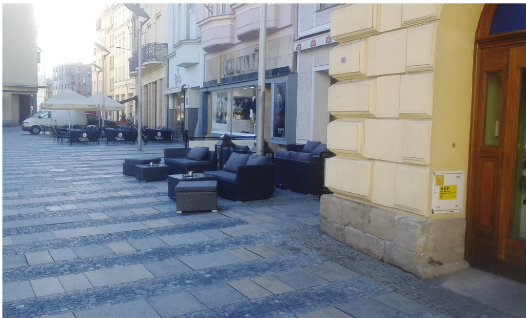
Fig.3: Placing a restaurant's furniture along a guide line, not protected by a compact element without an artificial guide line in the whole walking space (Masaryk Square, Ostrava).
