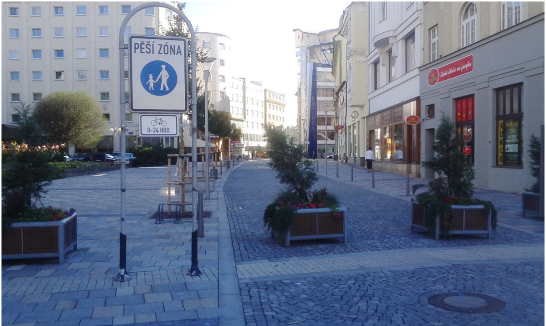
Fig.5: Unsuitably close placement of furniture in space without providing for a comprehensible walking strip, without any line orientation (pedestrian zone in 28. října street, Ostrava)
