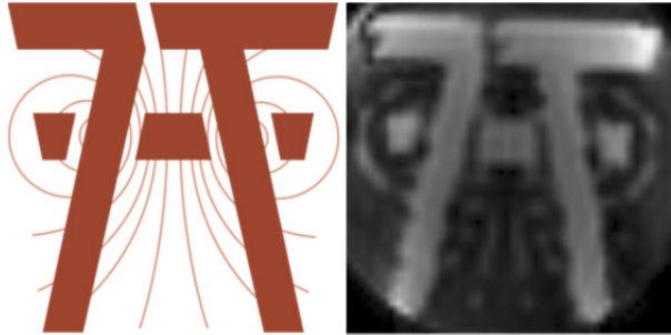
Figure 1.6: On the left the logo of the Erwin L. Hahn Institute for MRI is shown, on the right the pattern of the logo as excited in a spherical oil phantom using an 8-channel transmit/receive head array.
