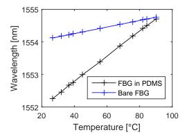
Fig. 9: Bragg wavelength dependence of non-encapsulated (blue line) and encapsulated (black line) FBG on temperature.
