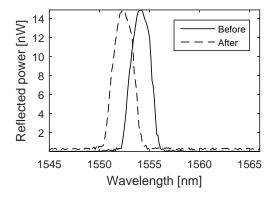
Fig. 7: The spectral characteristic of FBG before and after curing.
