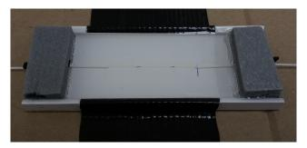
Fig. 5: Realization of encapsulation of FBG.
