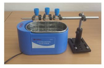
Fig. 4: Used ultrasonic bath for preparing Sylgard 184 mixture in the ratio 10:1.
