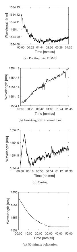
Fig. 6: Spectral characteristics of Bragg grating during encapsulation.
