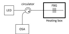
Fig. 3: Scheme of measurement with heating box.
