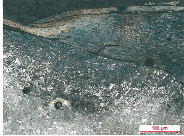
Fig. 3 The depth of cracks in sample 4A of the material collected from the bottom part of the track groove
