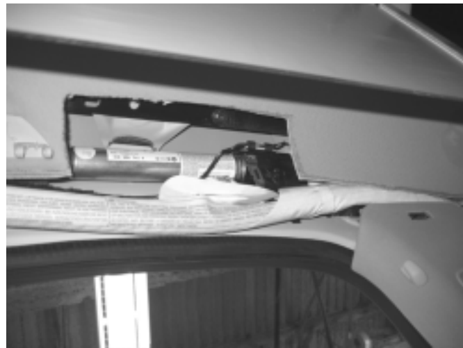
This photo shows the location of the gas cylinder for the side curtain air bag. The shot is from the inside of the vehicle with the "B" post showing just to the right of the cylinder.
