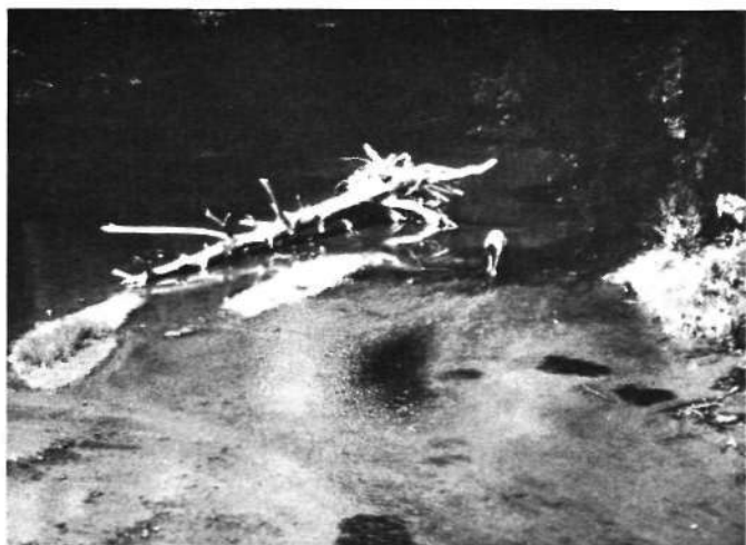
Figure 2. Dose of fluorescent dye appears as a dark discolorant to the flowing water (Photo courtesy M. D. Hale, U. S. Geological Survey, Indianapolis)
