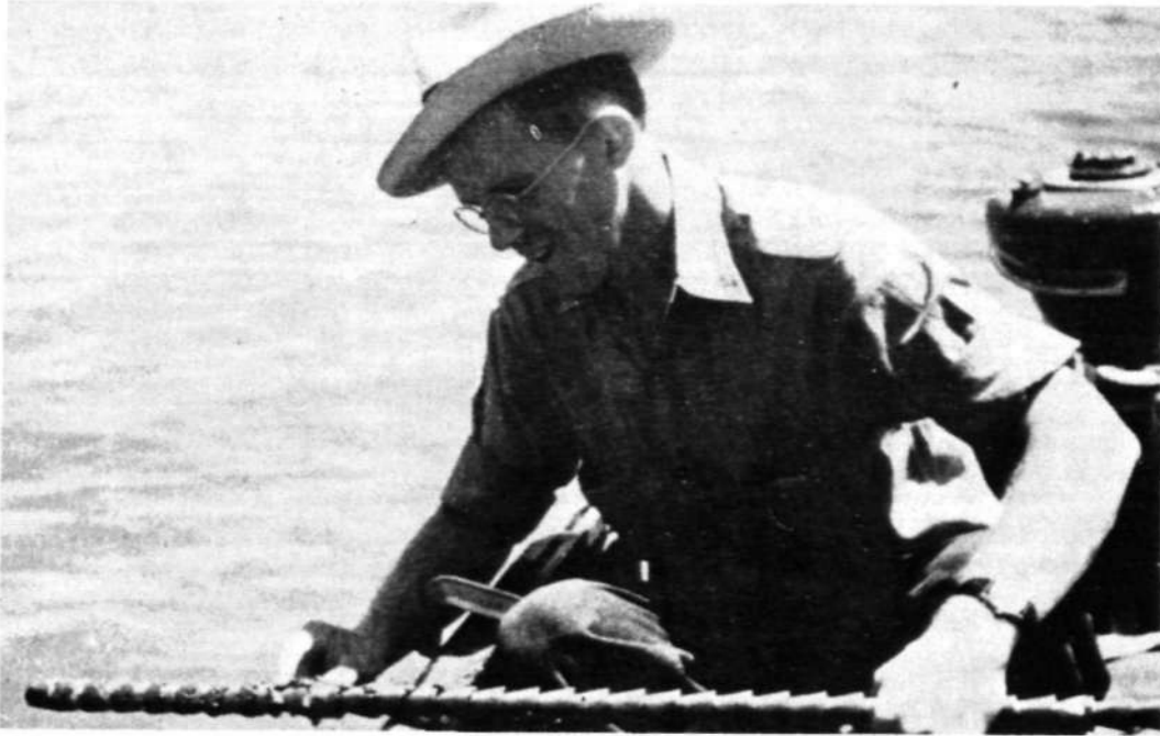
Figure 3. Use of the Spud in Measuring Silt Thicknesses.
