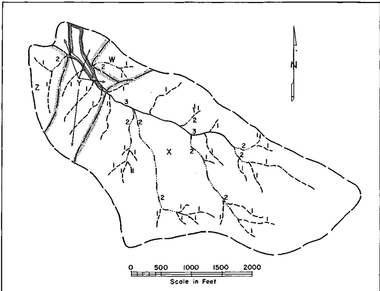
FIGURE 7 STREAM SYSTEM OF LAKE NO. 6 WATERSHED SHOWING HORTON ORDER NUMBERS AND FOUR DIRECT SUBBASINS
