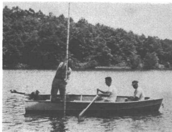
FIG. 4. USE OF SOUNDING POLE.
