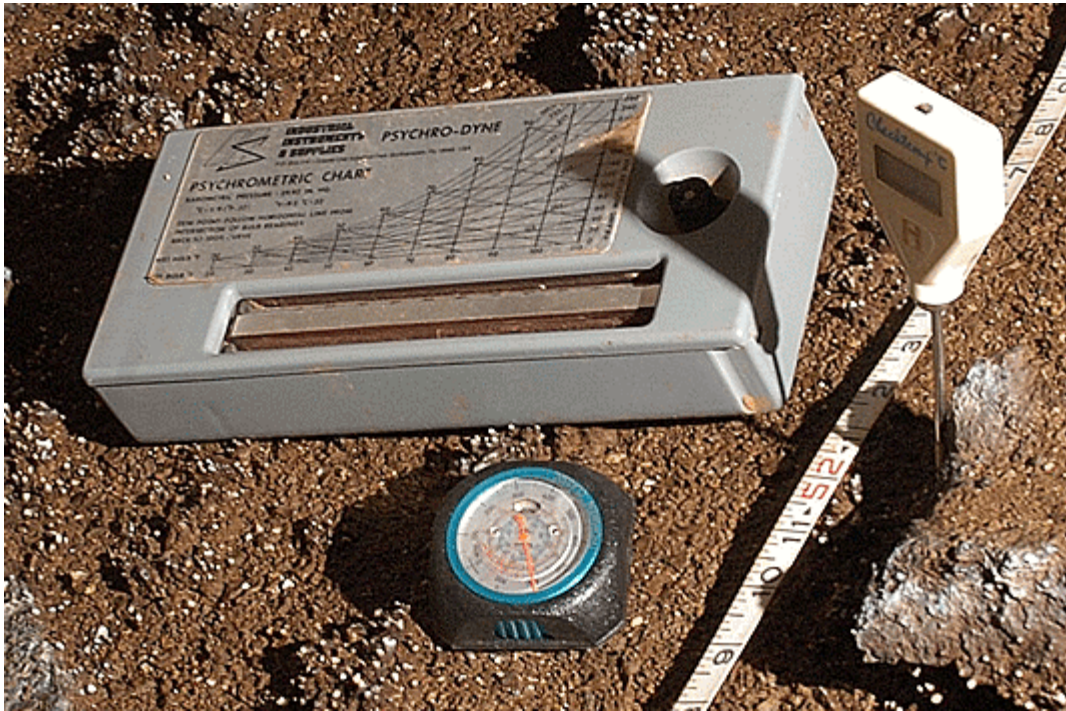
Figure 3. Psychro-dyne ® psychrometer (large gray box), soil temperature probe (white, on right side), and barometer (bottom) used to collect environmental data during the 2 June – 4 August 2005, lava tube bioinventory at Lava Beds National Monument, California. Photo by Jean Krejca.
