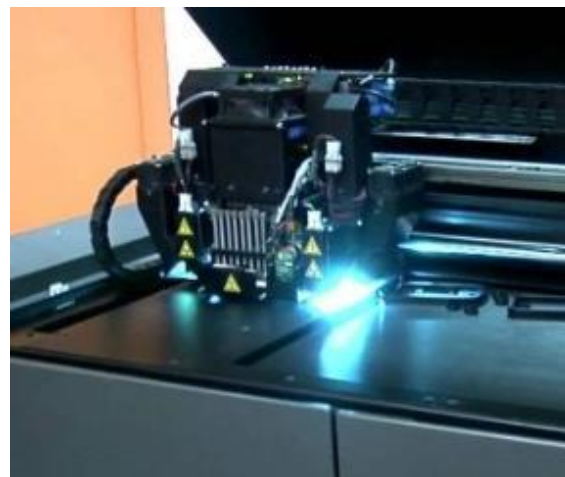
Figure 2.3.1: Material Jetting Process (Polyjet) www.3dnatives.com
