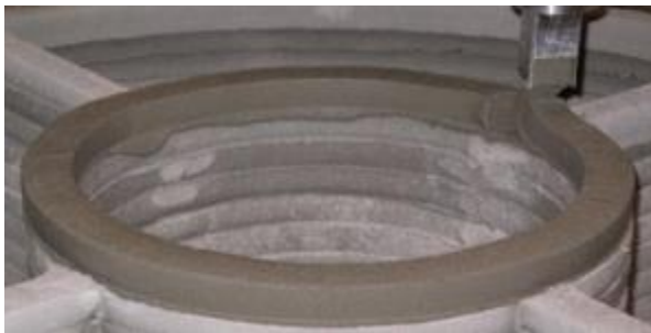
Figure 2.10.2: Contour Crafting In Operation archive.cooperhewitt.org
