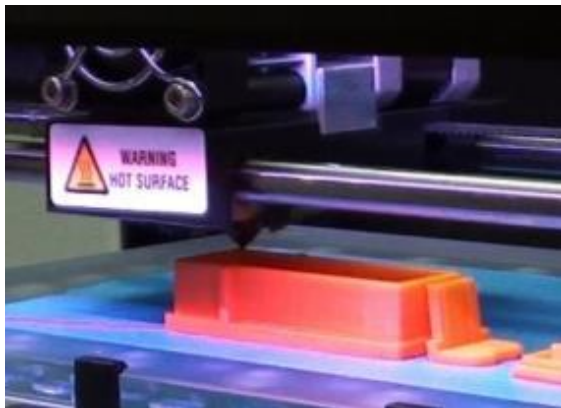
Figure 2.5.2: FDM Process www.inkfactory.com
