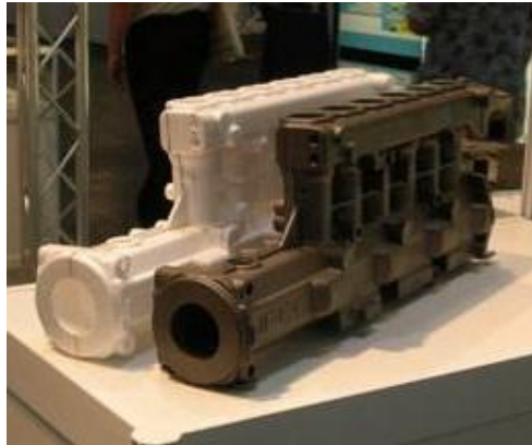
Figure 4.15.4: Lost Foam Casting and Master www.jmt.in
