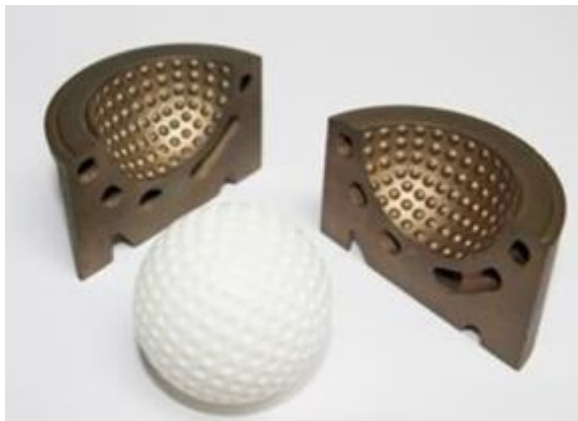
Figure 4.10.3: Tooling with Cooling Channels www.mmsonline.com
