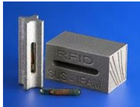
Figure 4.28.1: RFID Chip Embedded Into AM Part www.ineffableisland.com
