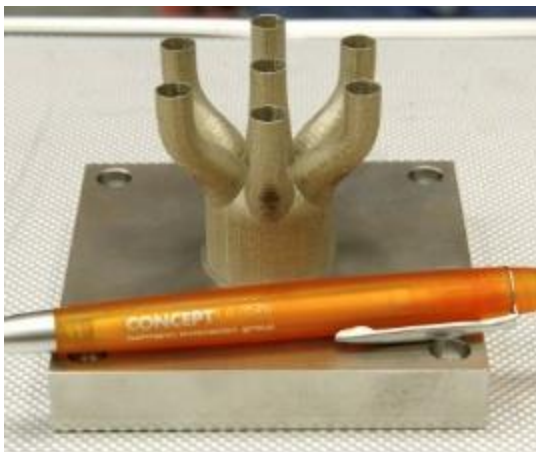
Figure 4.2.2: Complex Rocket Component Made By AM www.industrial-lasers.com
