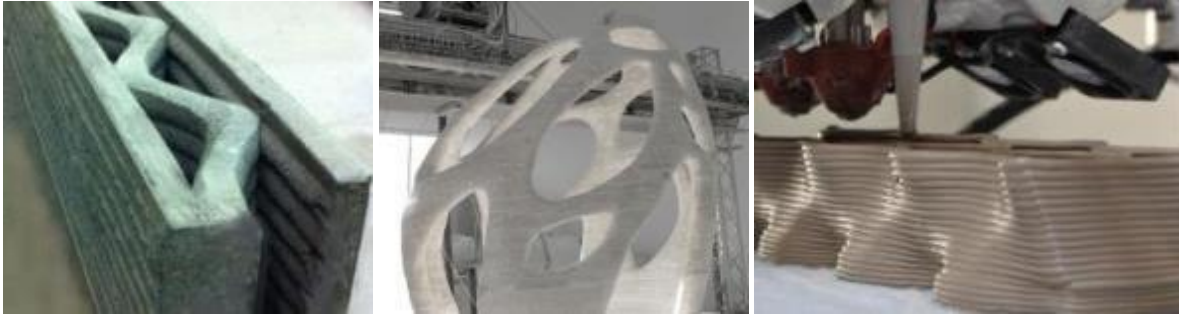
Figure 4.16.2: Products Made by Contour Crafting, D-Shape, and Concrete Printing www.dailymail.co.uk , openmaterials.org , blog.ponoko.com
