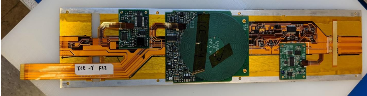
Figure 11: Flex Cable assembled with ADCS devices, and glued to the solar panel
