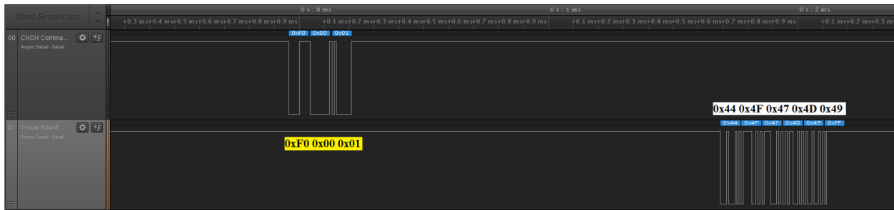
Figure 53: Power Board Responds to C&DH commands
