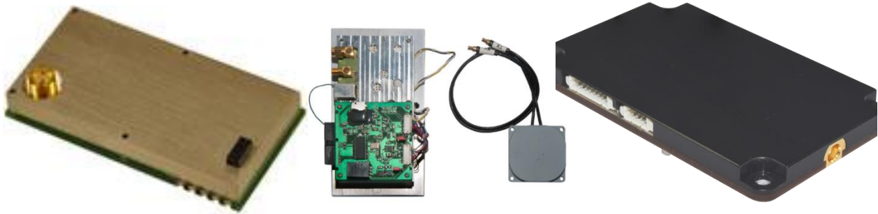
Figure 12: Radios Selected for IlliniSat-2: From left to right, AstroDev Lithium Radio, GlobalStar EyeStar D-2 Radio, GOMSpace NanoCom AX100 Radio
