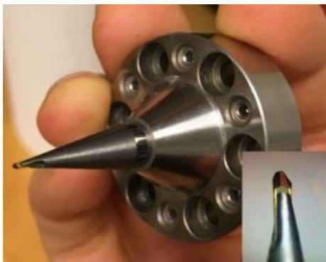
Figure 2.3: Chuck holding micro-milling bit [6]
