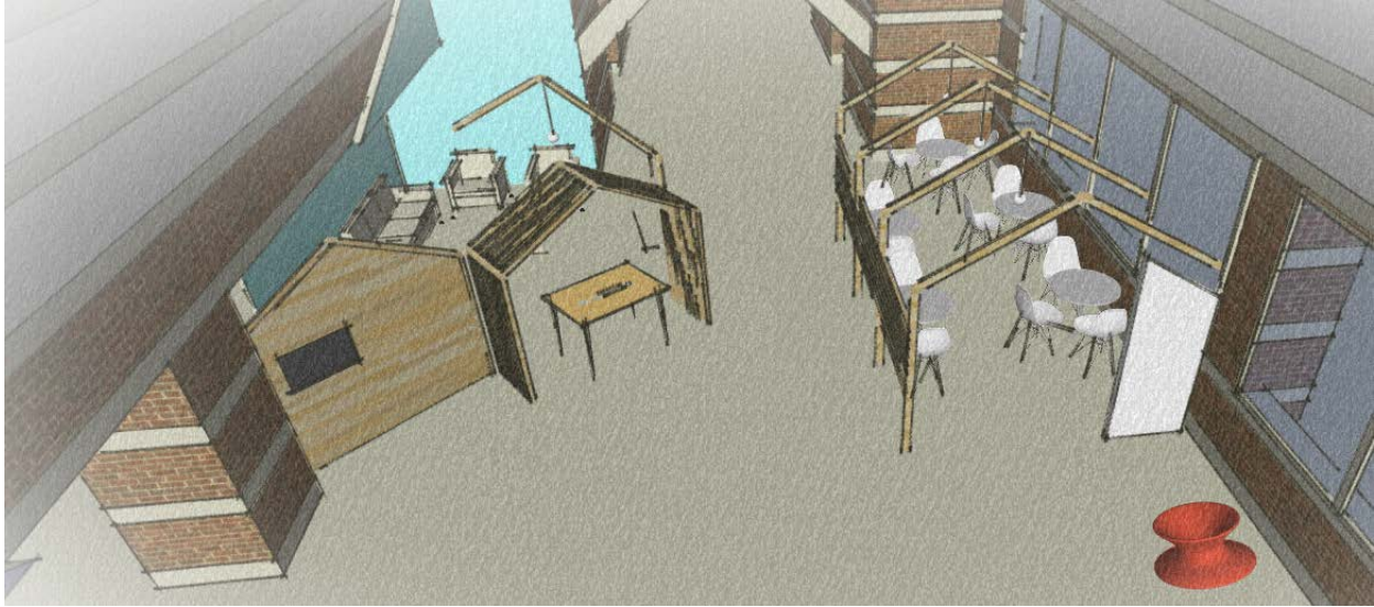
Figure 5.3: This image provides an example of how a pod structure may be incorporated into the future design of the Beckman atrium. This rendering is not final, as observations of the pod prototype currently installed within the atrium space will inform the eventual final design.
