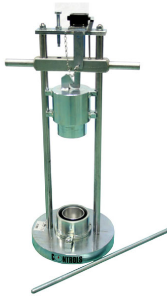
Figure 8: Impact test machine. Weight will be dropped from the top onto the testing specimen. Most studies focused on low velocity impact which is more common than high velocity impact
