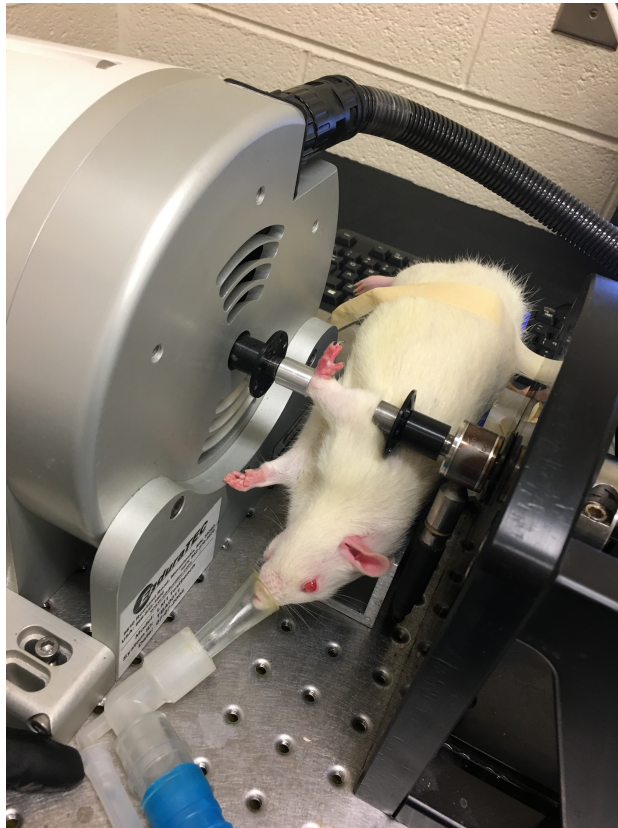
Figure 10: Cyclic load equipments consist of a computer, an actuator, and a load cell. It was important to secure the ulna into the caps. The concentration of the isoflurane should not exceed 3% for safety purpose.
