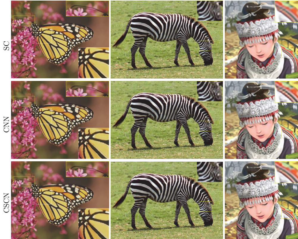
Figure 2.10: SR results given by SC [8] (first row), CNN [18] (second row) and our CSCN (third row). Images from left to right: the “monarch” image upscaled by \times 3 ; the “zebra” image upscaled by \times 3 ; the “comic” image upscaled by \times 3 .
