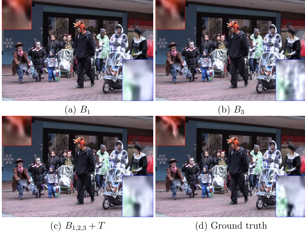
Figure 4.3: Examples of SR results from walk by 4x upscaling using different network structures. Compared with B_1 and B_3 , the temporal adaptive architecture B_{1,2,3} + T is able to effectively handle both the rigid motion shown in the top left zoom-in region and the complex motion in the bottom right zoom-in region.
