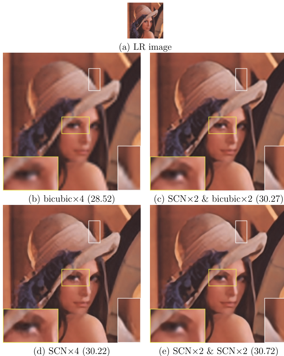
Figure 2.3: SR results for the “Lena” image upscaled by 4 times. (a) \rightarrow (b) \rightarrow (d) represents the processing flow with a single SCN \times 4 model. (a) \rightarrow (c) \rightarrow (e) represents the processing flow with two cascaded SCN \times 2 models. PSNR is given in parentheses.
