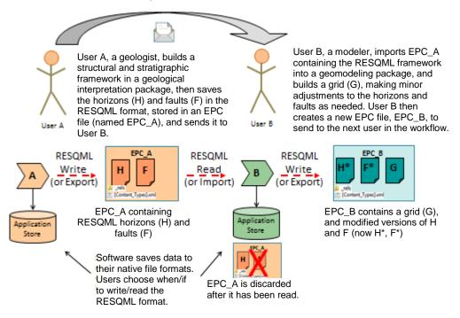
Figure 2. A user writes (exports) a file to the RESQML format, which is stored in an EPC file and may be read (imported) by other RESQML-enabled software.
