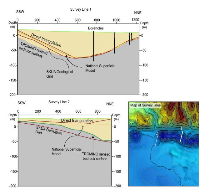
Figure 3. The results from the two passive seismic lines compared to the surfaces created by the different methods described in Figure 2. Survey line 2 shows that the apparent gap in the valley predicted by SDTM and the direct triangulation method is likely to be an artifact of the interpolation.
