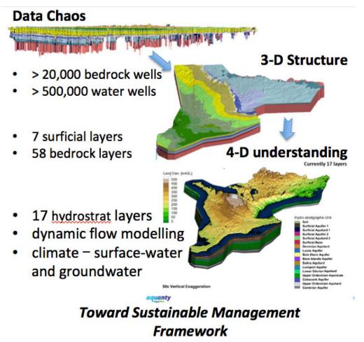
Figure 2. Transition in data framework from 2-dimensional point data (boreholes) to regional interpolated surfaces (geological model) to numeric groundwater model and groundwater knowledge framework.
