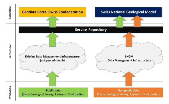
Figure 3. Schematic architecture of the SNGM, partly falling back to the existing data management infrastructure of the Swiss geodata portal.
