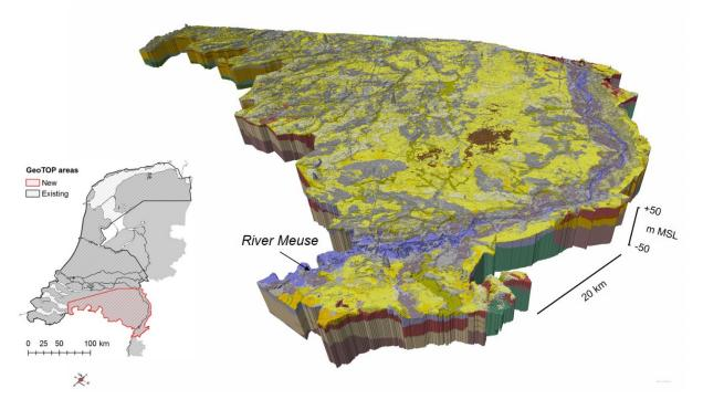
Figure 2. 3D view of the latest GeoTOP model area in the southeastern part of the Netherlands. The voxels are color-coded with stratigraphy. This part of the model was derived by voxelizing the upper part of the new, integrated national framework model that reaches down to  $\sim$ 500 m and has detailed stratigraphy (including many Holocene and upper Pleistocene formations, members, and beds) in the upper  $\sim$ 50 m.
