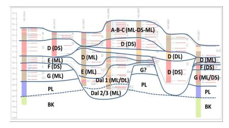
Figure 4. Geological interpretations based on fine-gravel analyses. ML: Clay till; DS: Meltwater sand; DL: Meltwater clay; PL: Palaeogene clay; BK: Danian Limestone. Figure from Sandersen and Kallesøe (2017). Fine-gravel analyses shown as background for the geological interpretations are from Andersen and Sørensen (2016).
