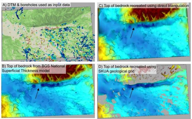
Figure 2. A) Distribution of borehole input data used in the test. B) Top bedrock surfaces from the current BGS superficial thickness model (SDTM). C) and D) The recreated surfaces using different methods. Note that only method D) does not contain the apparent (arrowed) gap in the buried valley.
