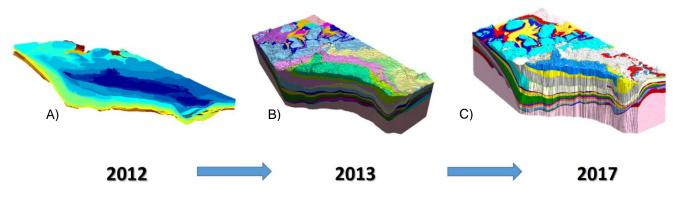
Figure 2. Development of the AGS Provincial Geological Framework model. A) In 2012, 35 2.5D provincial-scale grids were modelled, of which B) 19 geological units were modelled to create the first 3D provincial-scale geological model (version 0) in 2013. C) Provincial Geological Framework, version 1 was completed in 2017 and published online in 2018.
