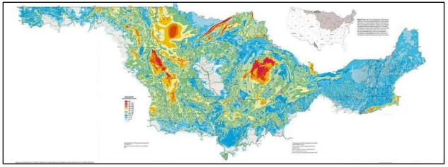
Figure 2. Sediment thickness map (above) (Soller and Garrity, 2018). Figure 3. Bedrock topography map (below) (Soller and Garrity, 2018). Both figures are example data to be included in the national 3D geologic framework database of the glaciated U.S., and have been modeled at a scale of 1:1,000,000 (reduced to 1:5,000,000 for publication, https://ngmdb.usgs.gov/Prodesc/proddesc\_106843.htm).
