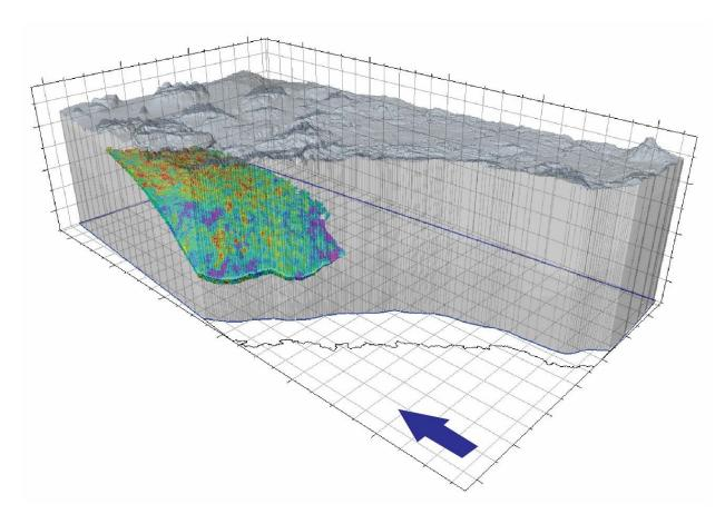
Figure 2. One porosity realization from the Montney 3D property model set within the 3D Provincial Geological Framework Model of Alberta (transparent gray and blue outline; province of Alberta outline in black) (vertical exaggeration of 50x).
