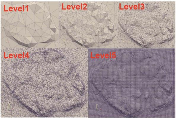
Figure 3. Five levels of generalization for a topography surface mesh feature.
