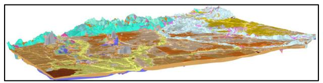
Figure 5. Regional geological model of the Vale of York looking northwest, with the Pennines in the background and showing the complex glacial and Holocene deposits in the foreground. (From Burke et al. 2017, supported by the Environment Agency.)
