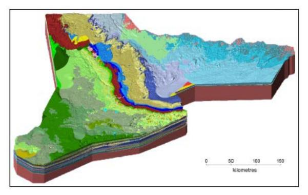
Figure 1. Southern Ontario bedrock model domain with subcropping–outcropping bedrock geology. Note the geology shown within the lake basins. Bedrock transitions stratigraphically upward from east to west, from Ordovician (blue, mauve) to Silurian (yellow, blue, brown) to Devonian (green).
