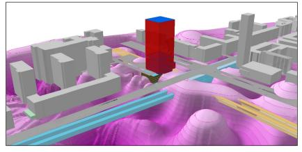
Figure 3. Shallow geological model of glacial deformations of Pliocene clays in Warsaw with two lines of the underground intersecting (courtesy Ryżyński G.).
