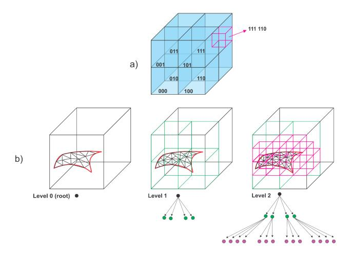
Figure 1. (a) Octree data structure and spatial indexing. (b) Variable subdivision of blocks.
