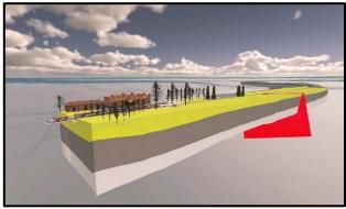
Figure 4. Example of BIM infrastructure design elements integrated with geological subsurface information, including faults. (BGS)
