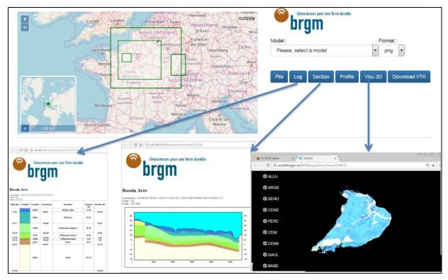
Figure 1. Representation of the Avre Basin geological model (Pennequin et al. 2017) in the web application using the generic interface and available services: knowledge geological architecture (geological pile), log, section/profile, and 3D visualization.
