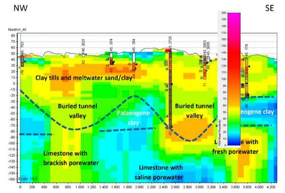
Figure 2. Conceptual cross-section through the study area. The coloured background is a 3D grid of resistivities from TEM data (transient electromagnetic data; resistivity scale to the right). Vertical rods are boreholes from the national borehole database Jupiter (red colours represent sand/gravel; brown is till; orange is meltwater clay; blue is Palaeogene clays). Vertical scale to the left is in meters above sea level and vertical exaggeration is 10 times.
