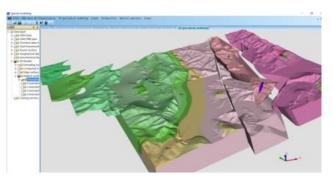
Figure 9. 3D geological map formed by the coupling modeling technique of implicit geological interface based on the grid field.
