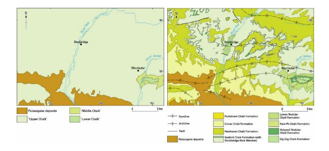
Figure 2. An example bedrock geological map (Winchester district, BGS 1:50,000 scale, geological sheet 299) showing the difference between the traditional classification of the Chalk (left), and the new detailed lithostratigraphy (right). Using the new lithostratigraphic mapping, faults and fold structures can be identified clearly.
