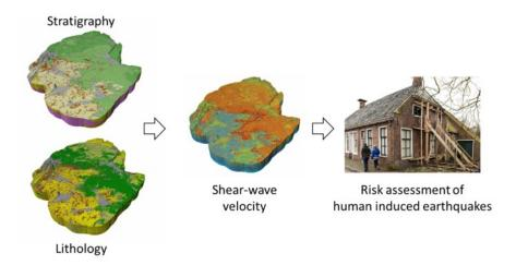
Figure 3. Putting the GeoTOP voxel model to work by adding properties related to the application at hand.
