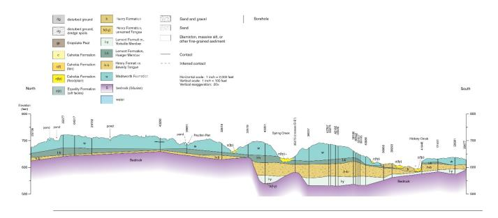
Figure 3. Schematic example of the bedrock valleys below Spring Creek and Hickory Creek showing how cross section building was used for data quality control and correlation.
