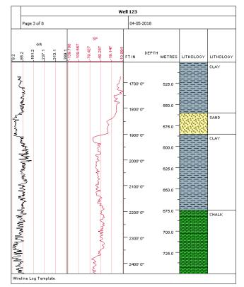
Figure 1. Groundhog Desktop borehole log, showing wireline log readings alongside traditional geological measurements.
