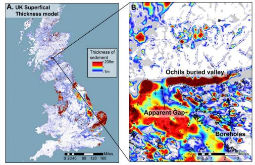
Figure 1. A) SDTM, the BGS national superficial thickness model. B) The Ochils buried tunnel valley as shown in SDTM. Black dots mark the positions of boreholes. The apparent gap may be caused by the interpolation method.
