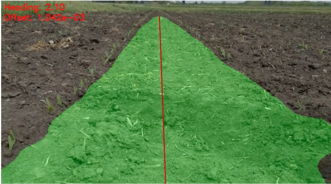
Figure 4.1: FCN detecting the row center and heading for vision based early-season navigation
