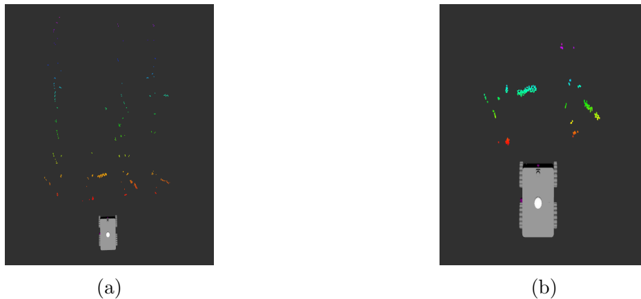
Figure 3.7: Laser scan cloud pre and post-filtering (a) Raw laser scan (b) Filtered laser scan showing the ROI
