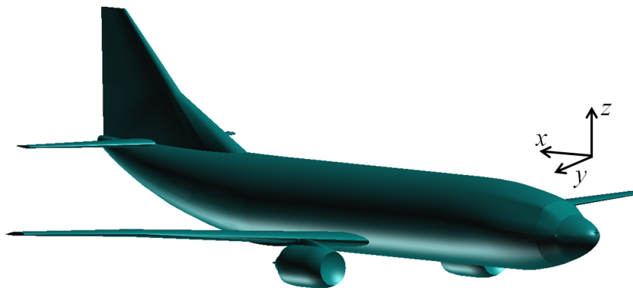
Figure 5.6: Geometrical configuration of the airplane model. The airplane has a body length of 35\lambda_0 and a wing span of approximately 38\lambda_0 . The ABC is placed 3\lambda_0 away from the nearest parts of the airplane, thus creating a total computational domain having a size of 41\lambda_0 \times 44\lambda_0 \times 17\lambda_0 .
