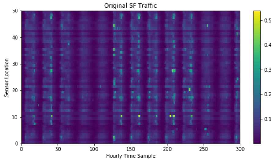
Figure 5.3: Original traffic data [10] - vertical axis shows spatial position of sensors. The horizontal axis represents hourly time sample indices. The pixel intensities indicate the level of traffic intensity, brighter color showing greater traffic and darker colors meaning lighter traffic
