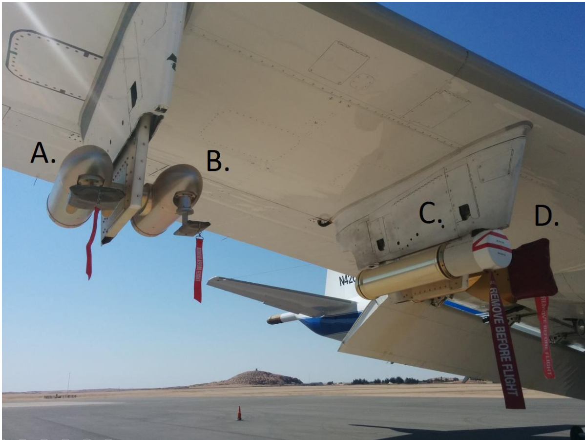
Figure 1: (A) CDP (B) King hot-wire (C) 2D-S and (D) HVPS3 mounted under the right wing of NASA P-3.
