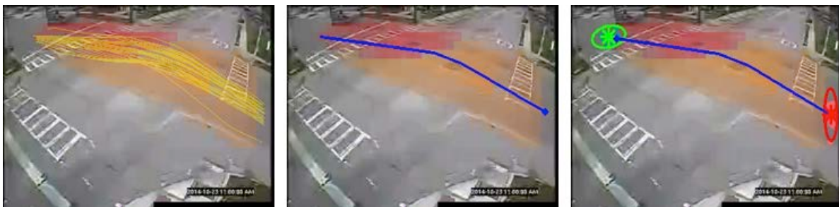
Figure 2: Ridges (left), centerline (middle) and entry exit (right) extracted by our algorithm.
