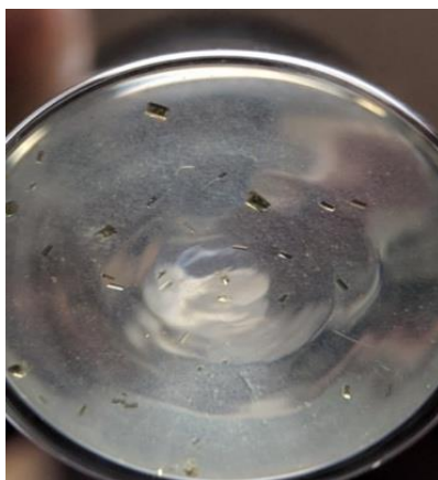
Figure 5. Pure phase KSU-1 yellow prismatic crystals. White powder is DPG that crashes out of solution. It can be removed by several DMF washes.
