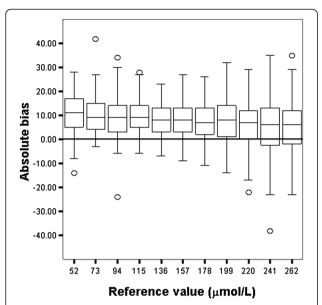
Figure 3 Box and whisker plot showing the absolute bias ( $\mu$ mol/L) for the Jaffe technique. The box represents the 25<sup>th</sup>, 50<sup>th</sup> and 75<sup>th</sup> percentile; the whiskers represent the 5th and 95th percentile. The extremes, defined as values more than three times the interquartile range, are the signs above and underneath the whiskers. The grey line represents the 0  $\mu$ mol/L bias line.
