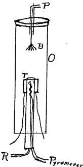
The larger outer portion 0 was a piece of glass tubing 4" in diameter, the top of which was closed with a large rubber stopper paraffined in. B was a brush of small iron wire as before suspended directly over the porcelain tube T which was wound with resistance wire at the upper end and this in turn covered with heat insulating material. The catalyzer was placed in the upper end of this
