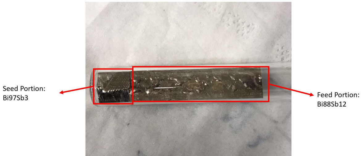
Figure 10: Seed and Feed portion before Zone Melting
