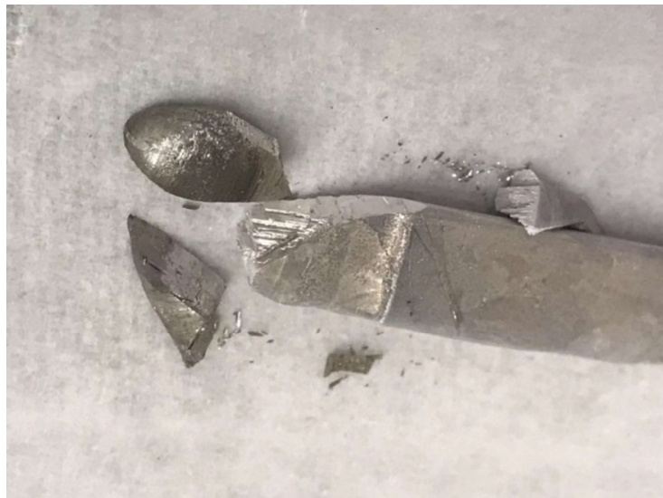
Figure 20: Single-crystalline \text{Bi}_{88}\text{Sb}_{12} alloy with 1% CuBr Dopant
