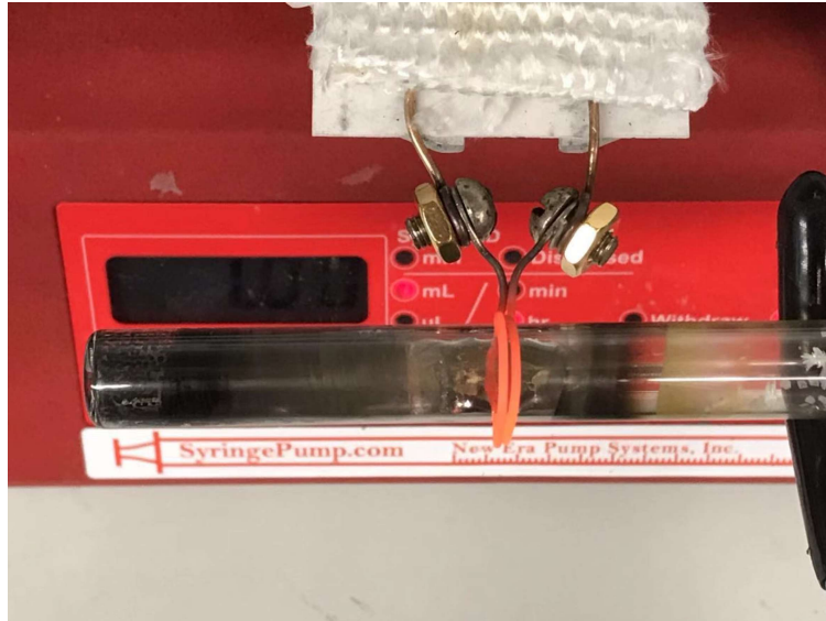
Figure 8: Zone Melting Method
