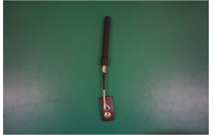
Fig. 3. The wireless passive SAW delay line temperature and pressure sensor node with antenna connected.
