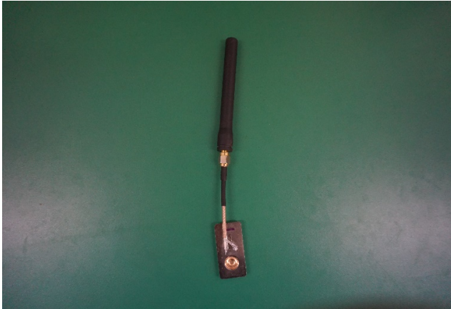
Fig. 2. The photo of wireless passive SAW delay line temperature and pressure sensor node with antenna.
