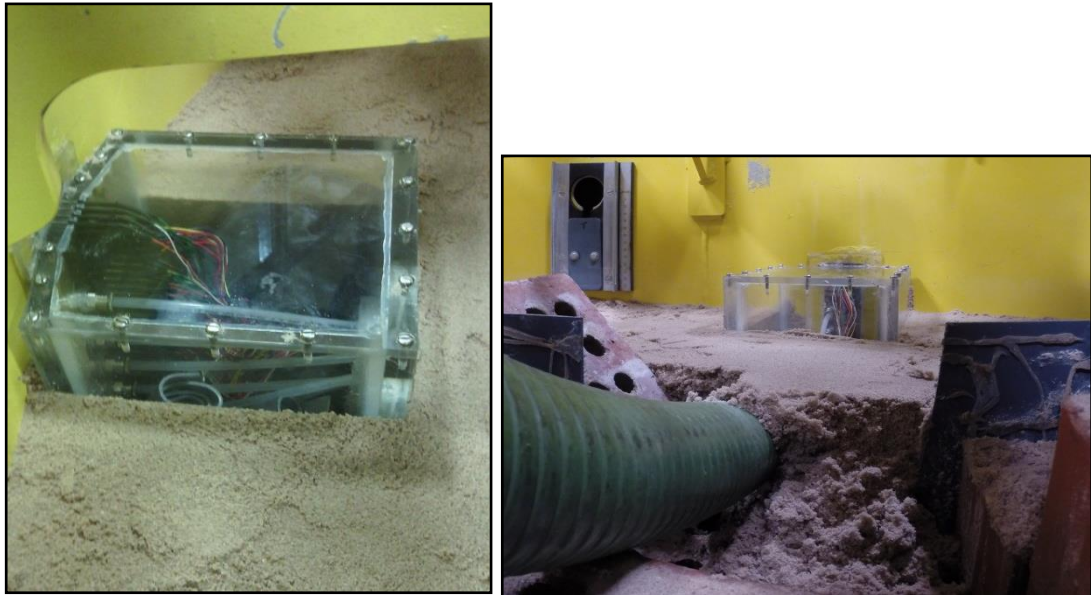
Figure 3.20 Images showing the Resistivity box being buried and fitted into the bed and flume prior to the erosion test.
