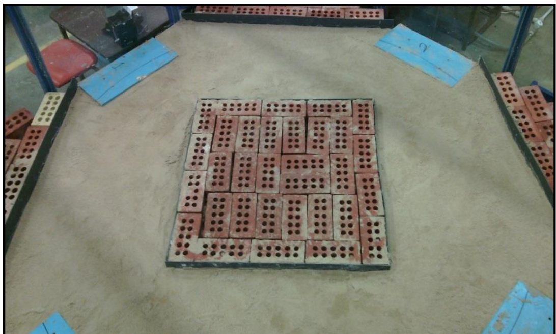
Figure 3.14 Image showing 100% sand bed prior to wetting and placing of annular flume
