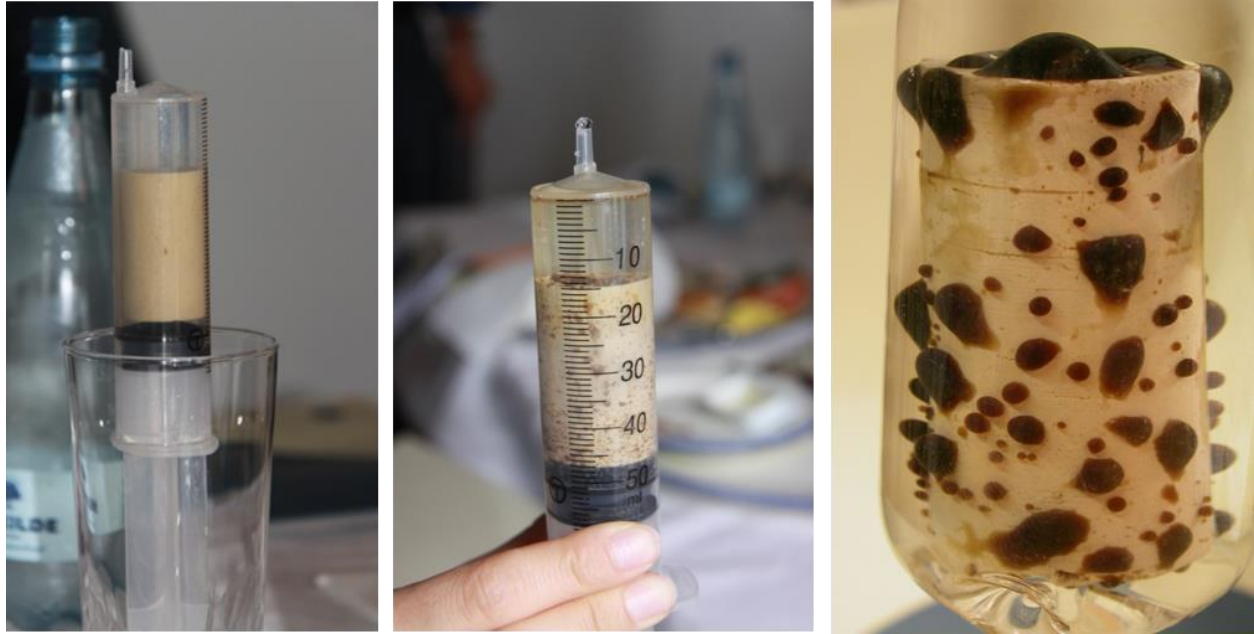
Figure 2.8: Imbibition experiment was carried out on chalk cores in the Ekofisk field showing the water wet chalk shows absorption of water quite effectively at low in situ water saturation (ConocoPhillips internal report).
