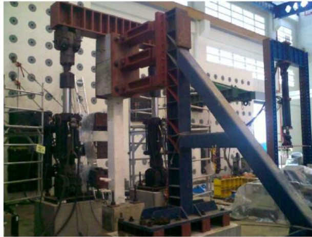
Figure 2.31. Hydraulic actuators at the Protective Engineering Laboratory in Nanyang Technological University, Singapore [120]
