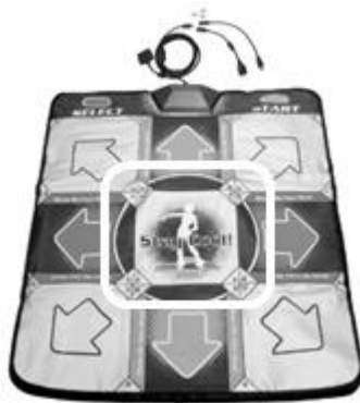
Figure 12. Floor mat with neutral square boundary highlighted
