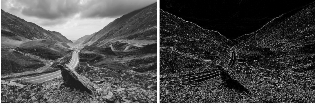
Figure 2.8: An example convolution of an image with an edge detecting kernel. Left shows the original image and right shows the feature map after convolution with a filter containing the values: \begin{bmatrix} -1 & -1 & -1 \\ -1 & 8 & -1 \\ -1 & -1 & -1 \end{bmatrix} .
