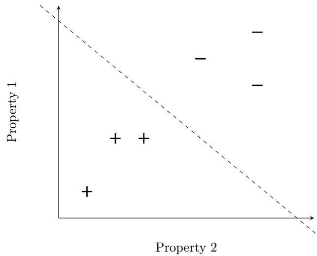
Figure 2.1: An example dataset containing instances split into two target classes. Each axis represents a feature. The dataset is homogeneously split by a linear hyperplane.
