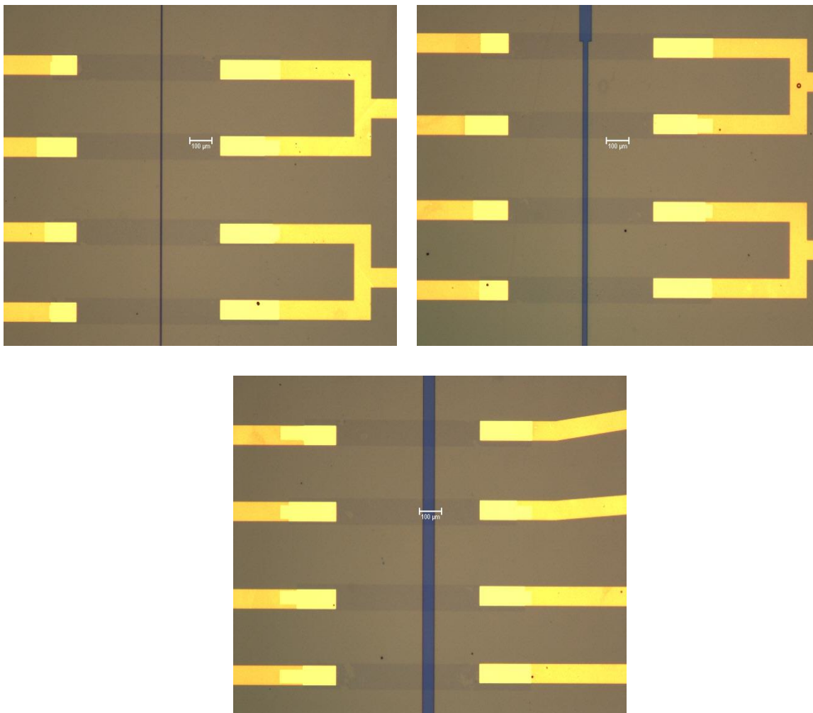
Figure 3.18: Optical images at 5x magnification showing flow channels of 3 different widths. Top left - 5µm, Top right- 20µm and Bottom left - 50µm. For all three images, the scale bar indicates 100µm
