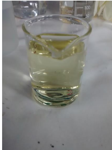
Figure 5.6: A photograph taken 1 minute after HRP-PBASE functionalized graphene is immersed in an OPD solution with Phosphate citrate buffer. The colourless solution turned yellow.
