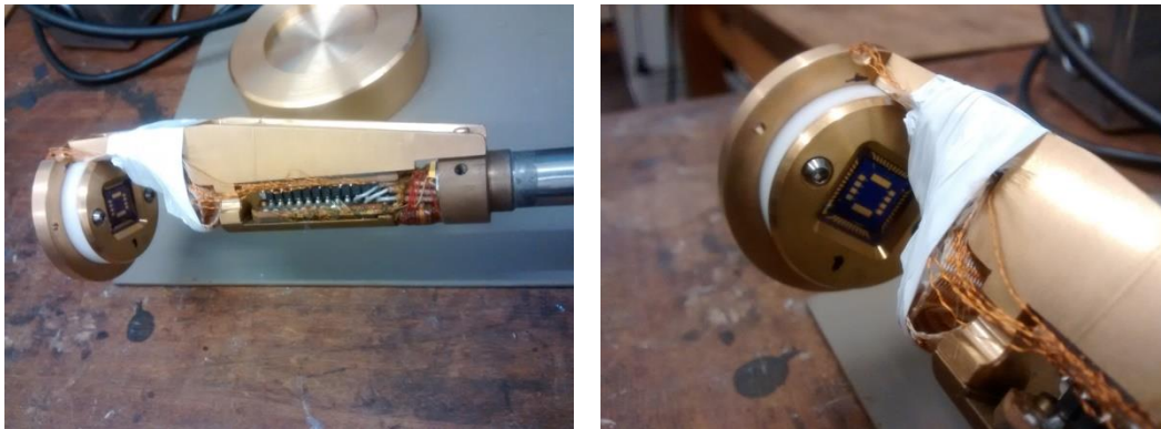
Figure 5.4: Substrate holder for the chip package Left: Side view showing wired connections to a port that is interfaced with a dipstick for low temperature measurements. Right : Top view showing the device architecture.
