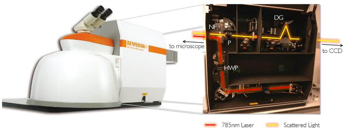
Figure 2.9: Renishaw InVia Raman microscope. The insert shows the beam paths of the 785 nm laser (red line) to the sample in the enclosed microscope, and of the scattered light (yellow line) through the optical components of the spectrometer to the CCD [HWP: half-wave plate; NF: notch filter; P: analyser (half-wave plate and polariser); DG: diffraction grating]. Adapted from: [1]
